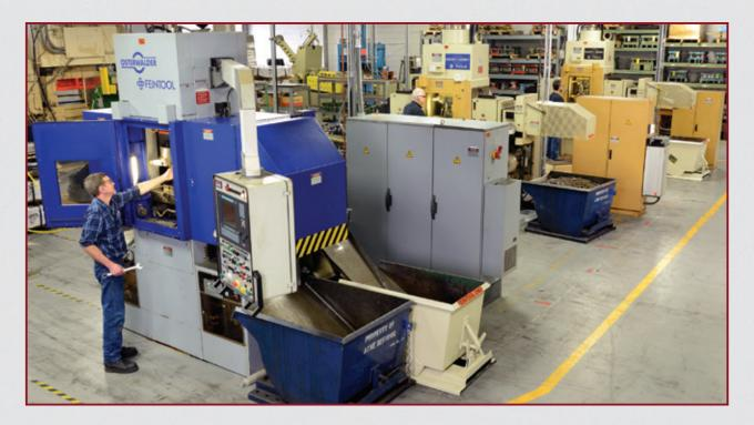
Sko-Die's fineblanking capabilities, expertise and Feintool presses deliver precision components with cleanly sheared surfaces over the entire material thickness in a single operation. Tolerance range is traditionally within one one-thousandth of an inch. Fineblanking provides production cost savings by maximizing efficiencies and eliminating secondary operations.
